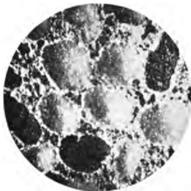
FIG. 42. — Photomicrograph of Cement-Ottawa Sand Mortar, showing Large Voids.
